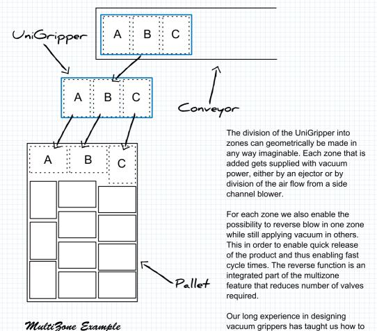
vacuum grippers has taught us how to make optimized zone divisions for each handling project. By analyzing the products that are to be handled and how they will be released, the number of zones can be optimized to provide the required versatility in the most cost efficient way.
